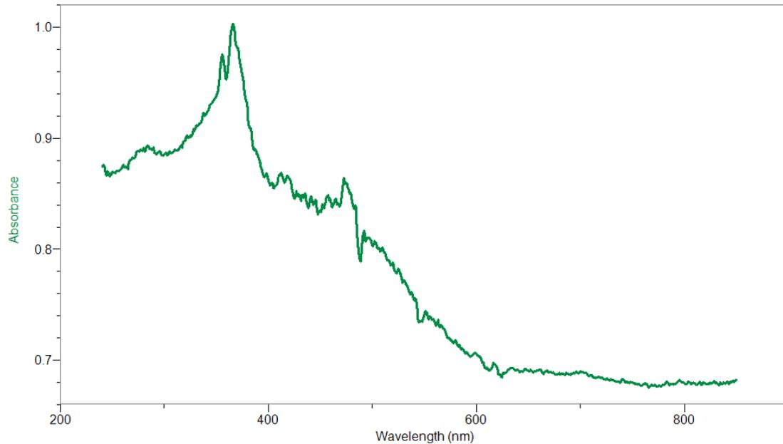
Figure 1. The UV-Vis absorbance spectrum of zinc oxide nanoparticles from 240 nm to 850 nm.
