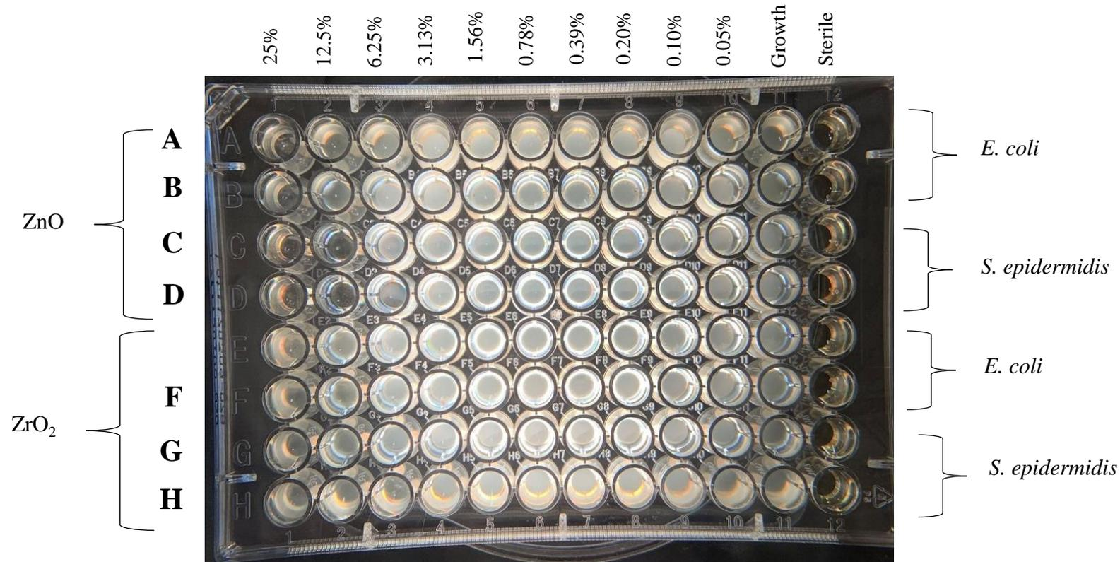
Figure 5. Minimum inhibitory concentration (MIC) Fall 2019 results for ZrO<sub>2</sub> and ZnO nanoparticles against *E. coli* and *S. epidermidis*. The initial ZnO and ZrO<sub>2</sub> NP concentrations were 72.5 mM and 83.6 mM, respectively.
