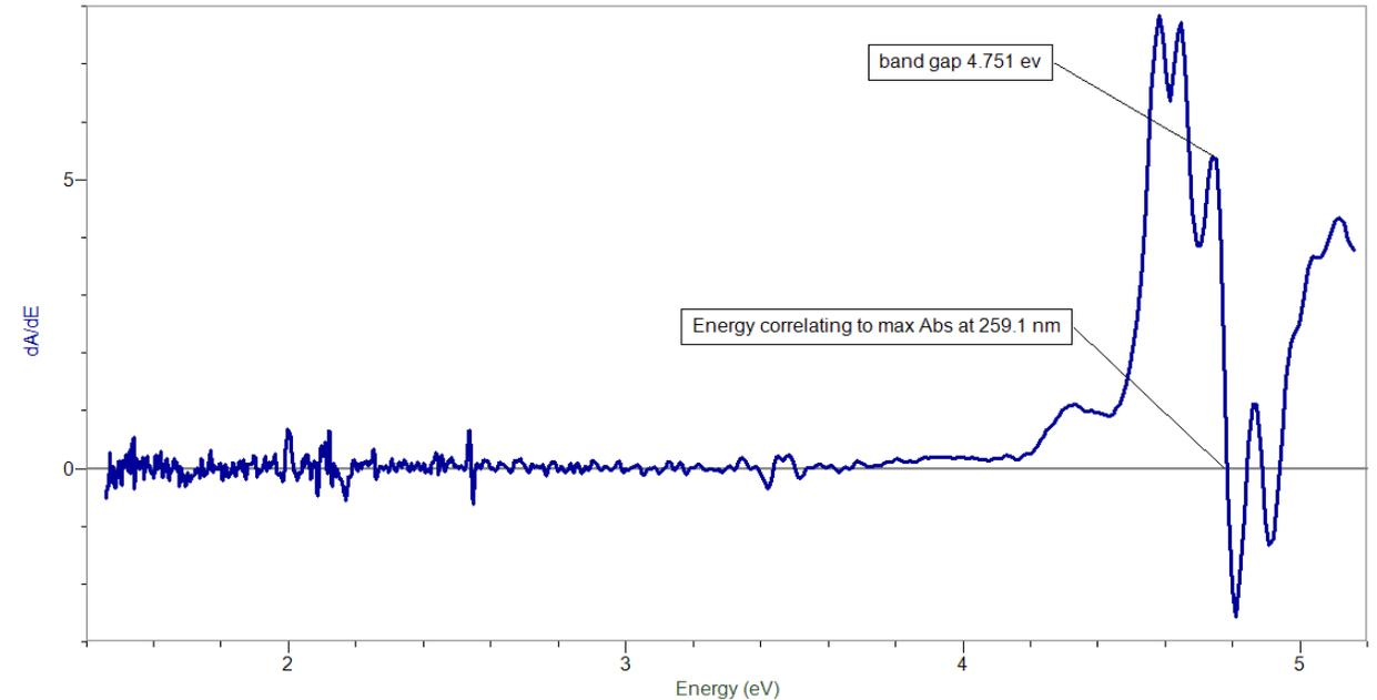
Figure 4. Zirconium oxide nanoparticles' first derivative of the absorbance spectra with respect to energy  $dA/dE$  in electron volts (eV).
