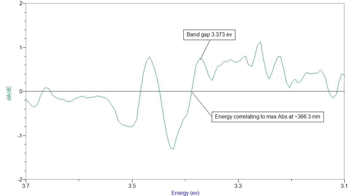
Figure 2. The first derivative of the zinc oxide nanoparticles' absorbance spectra with respect to energy  $dA/dE$  in electron volts (eV).
