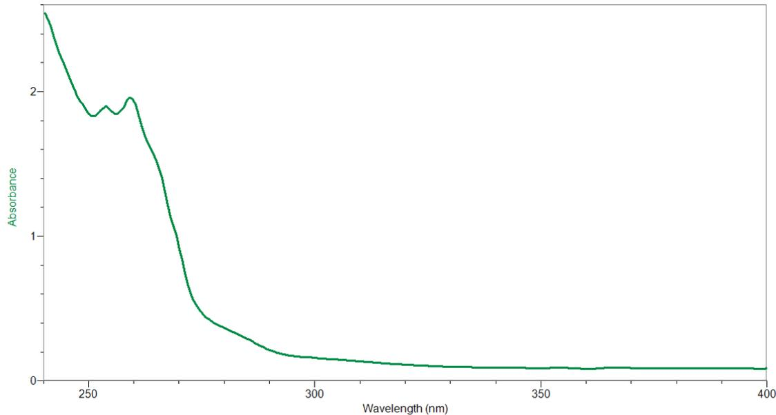
Figure 3. Zirconium oxide nanoparticles' UV-Vis absorbance spectrum from 240 nm to 400 nm.
